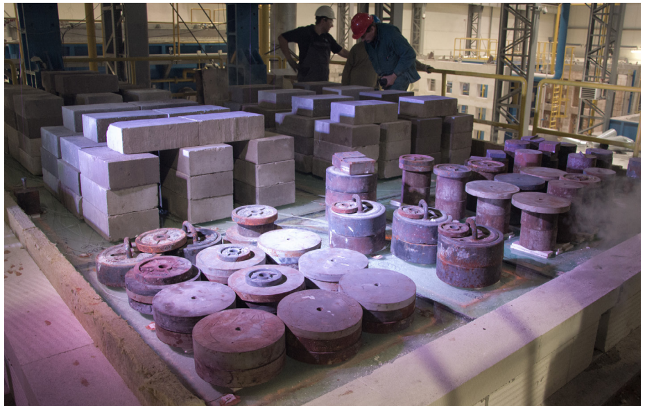
In the photo: ceiling with Polflam glass above the chamber of the testing furnace tested at the certifying body for resistance to fire. The structure of the ceiling contains glass panels of various dimensions and shapes that have been loaded in compliance with the load-bearing requirements of the technical standard.
