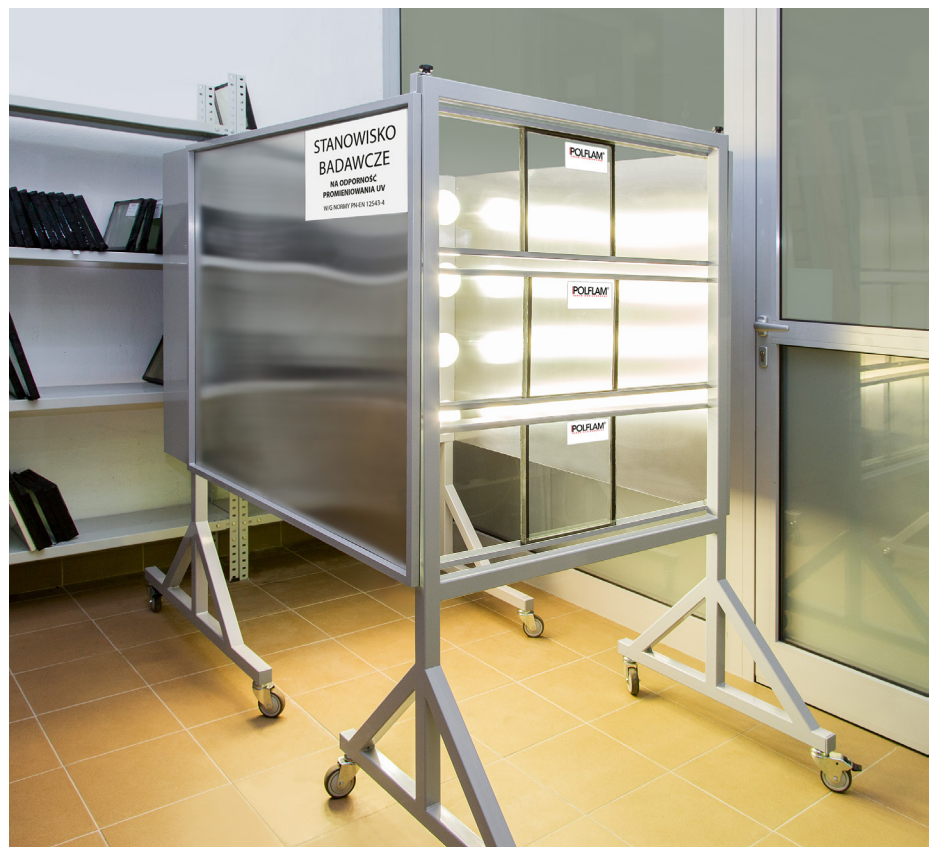
In the Polflam laboratory the glass is exposed to UV light.
