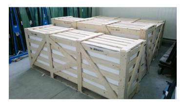
Glass panes can be packed in wooden cases with free sides, in accordance with the binding standards.
