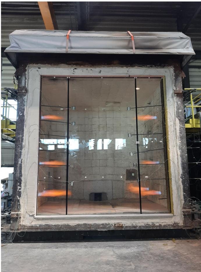
*When exposed to high temperatures, POLFLAM fire-resistant glass changes its structure and appearance, while retaining its shape. This serves as a solid barrier against fire and thermal radiation for over 120 minutes. Our glass successfully passed the test, significantly exceeding the time required for classification. ▶*
