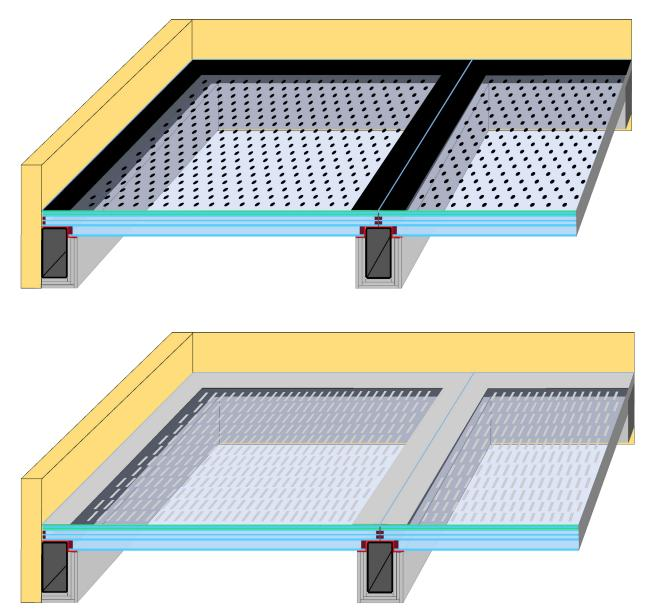
POLFLAM F glass is provided with an opaque edge screen printing  $\geq$  50 mm to conceal the supporting structure of the floor system.
